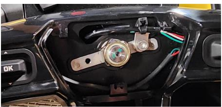
With a 10mm wrench, install the zip tie tab onto the threaded hole right of the steering wheel nut using the included M6 bolt and washer. Secure the OEM wiring to it keeping it as far from the steering wheel locking tabs as possible (circled in step 9).
