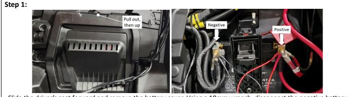
Slide the driver's seat forward and remove the battery cover. Using a 10mm wrench, disconnect the negative battery cable from the battery.
