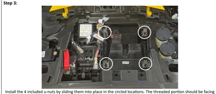
4 included u-nuts by sliding them into place in the circled locations. The threaded portion should be downward.
